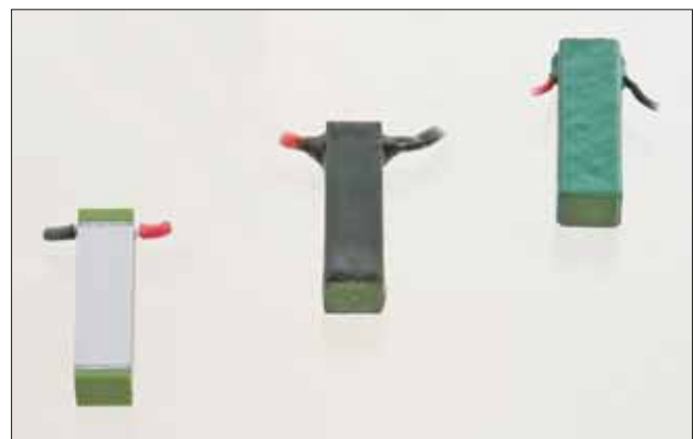
Fig. 3: Different kinds of stack coatings
