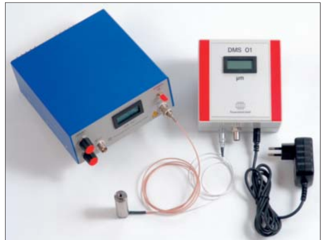
Basic position control equipment. Piezo-actuator with strain gage position sensor. Position read out by DMS 01 unit. Piezo-actuator supply electronics SVR 150 (left).
