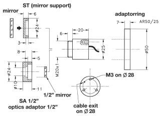
Piezo mirror-shifters are used for ultrafine axial positioning of mirrors and other optical components with out the use of heavy stages or other external guiding mechanisms.
